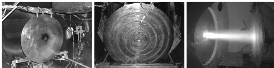
Fig. 8 Front and aft side of the baffle plate and during an experiment.
